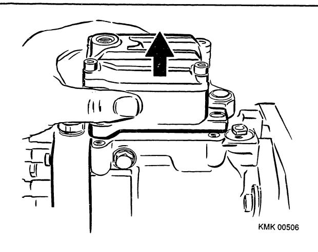
Unscrew electric shutoff device (ELAB). Visually inspect strainer of quantity actuator.
